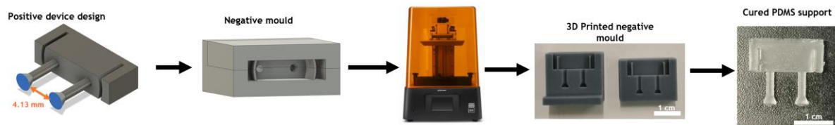
Figure 12 Representative images of positive and negative moulds and the final PDMS support.
