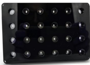
Picture of the SUP interface, equipped with 24 MUSbit™ chips
